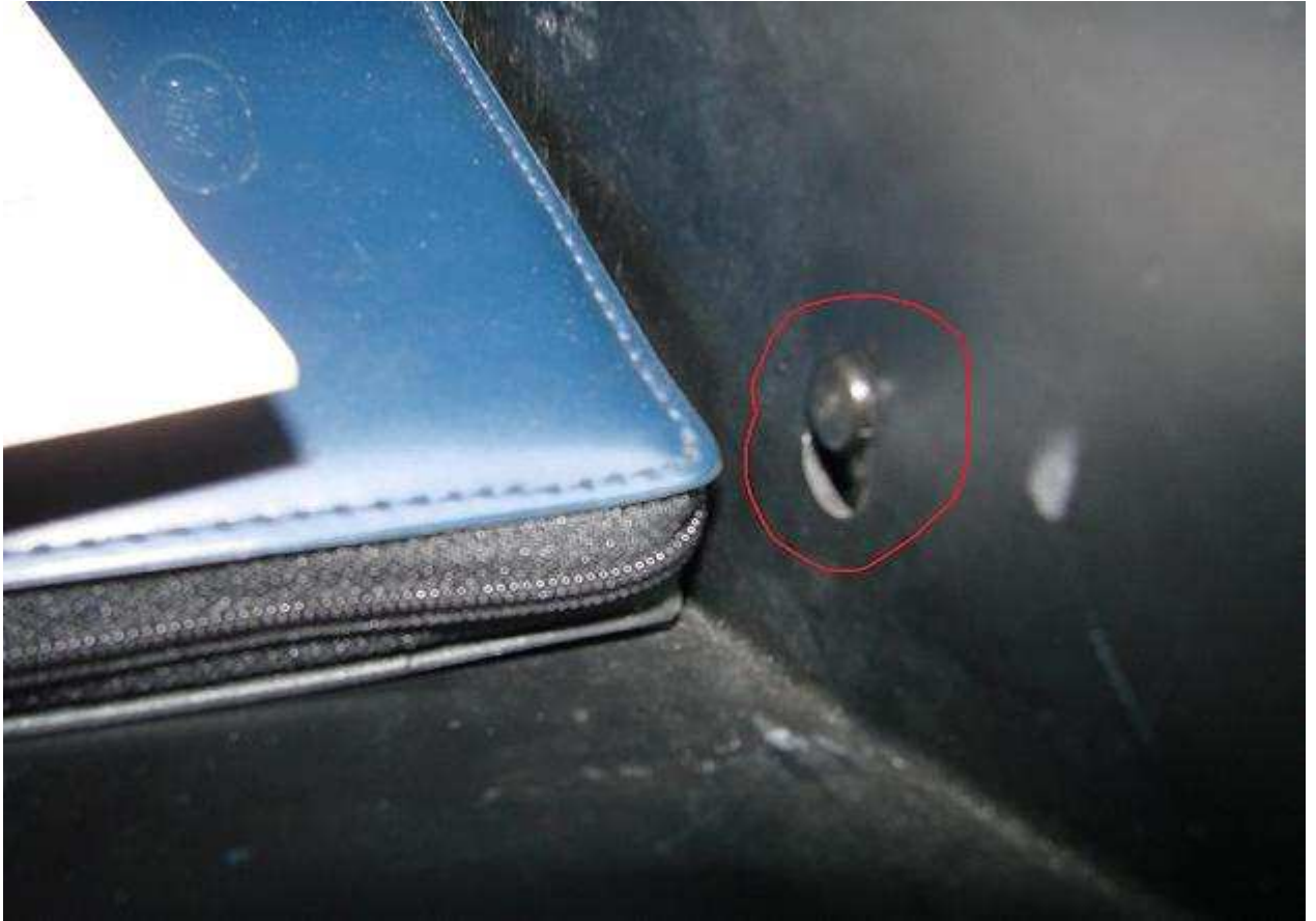
23. Another picture of the hook from the back side. See how it just slides down to the bigger hole.
