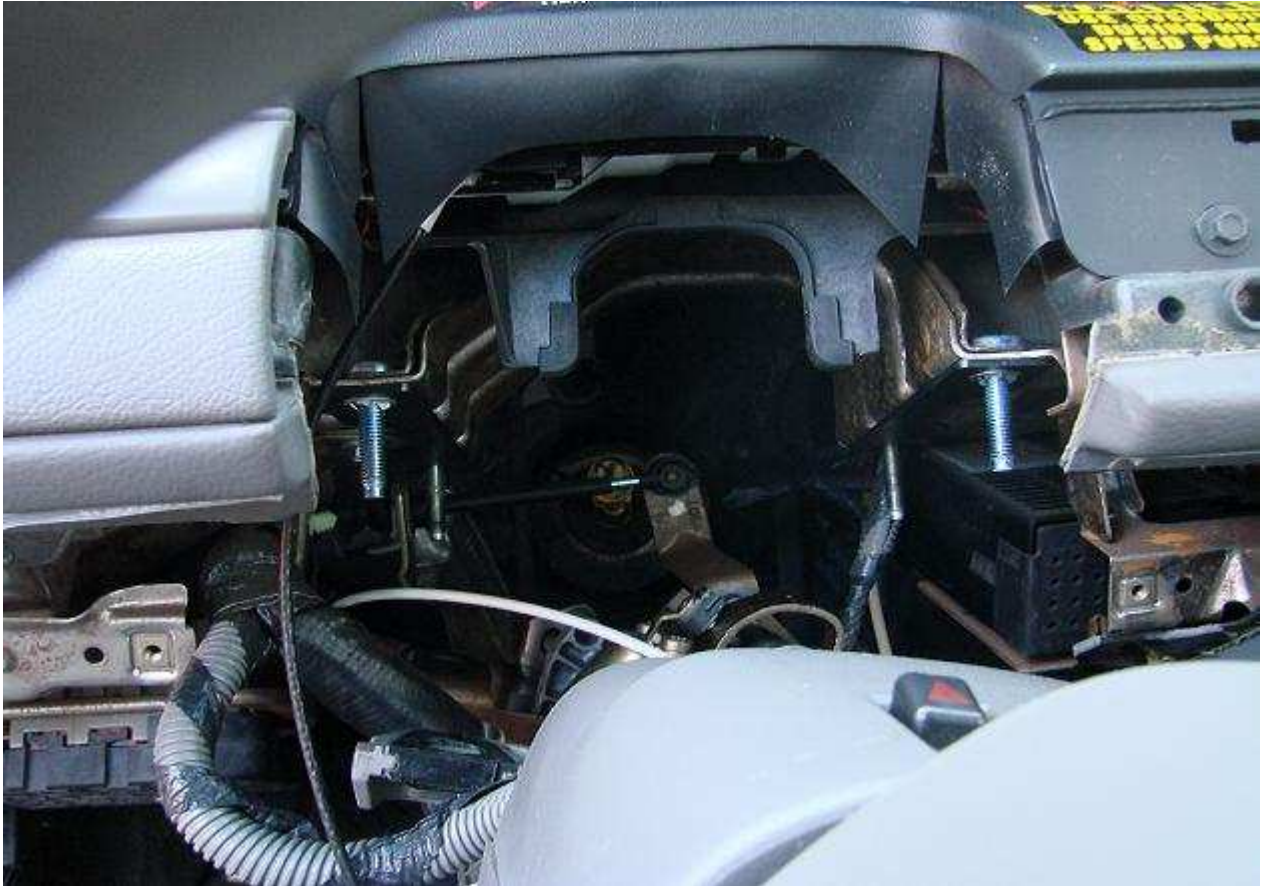
16. ) Here is a close-up of what the dash will look like when the column is dropped. There is no need to remove the column from the vehicle; this will allow plenty of room. From here you will see the fuse box to the left, and the LCM to the right (black vented box).
